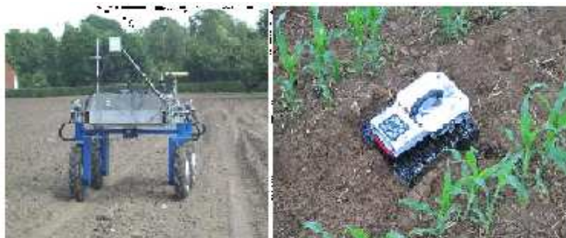
Figure 1: (Left) Portal Crop Scouting Platform (Madsen and Jakobsen 2001), (Right) Sub Canopy Robot ISAAC2
